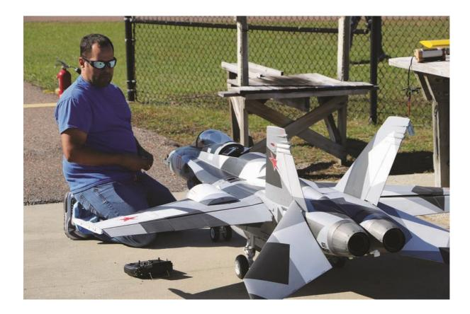
This Skymaster F-18 Hornet uses the flight mode setup on the PowerBox Core radio to activate several flight modes, including a landing mode that uses the elevators as ailerons for increased low-speed roll control along with a speed brake and gyro control.
