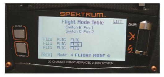
A Spektrum DX20 has a table where you can visualize what flight mode is active with each switch position. In this case, SWB controls the row and SWG controls the column for nine total flight modes. A very powerful system! (*NOTE: Many other systems are just as, if not more, powerful than Spektrum – Ed.*)
