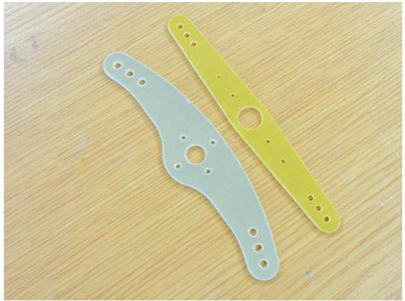
An offset arm as well as a straight arm for pull-pull. Using a straight arm is beneficial whenever the control horn on the control surface is directly in line with the hinge-line. Both arms shown above are to be bolted to a standard plastic or metal servo arm before being secured to the servo.
