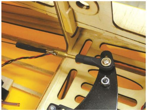
Shown here is an offset arm that is connected via a pull-pull system to the rudder control horn, which is also offset from the hinge line.
