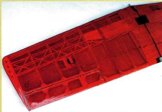
A view from the top of the left wing panel shows only one aileron is used, and its servo is installed internally. Note the extensive use of truss-type construction, which provides a lot of strength.
