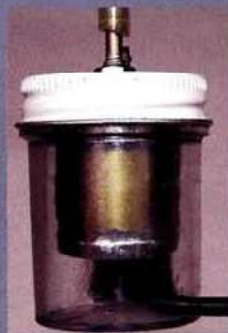
Maynard's home-made float chamber is pure simplicity: a plastic jar, some sheet brass and a no. 40 drill bit.
