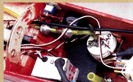
An overall view of the nose compartment. From left: on/off switch, backup battery, float chamber, C&H ignition module, carb and alternator. The throttle servo is mounted under the ignition module.
