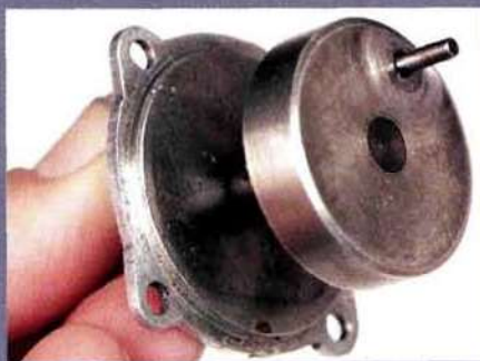
A close-up of the link that connects the alternator to the crankshaft. The pin inserts into the crankshaft.
