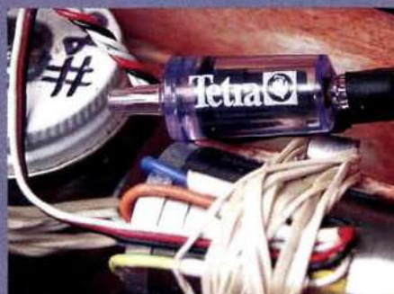
The one-way valve used to pressurize the fuel cell. It was designed for use in aquariums.
