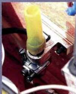
A close-up of the remotely mounted carb. Maynard modified the barrel to get the maximum efficiency needed for the flight.
