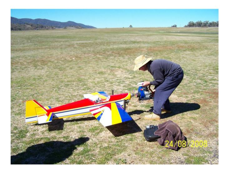
The starter was made from a 4 stroke 96 cc garden edging machine. As you can see from the next photo, he restrains the model with a special bar, which is seen lying in the foreground. The bar fits behind the undercarriage, attached to the wing restraints, when used for solo starts.
