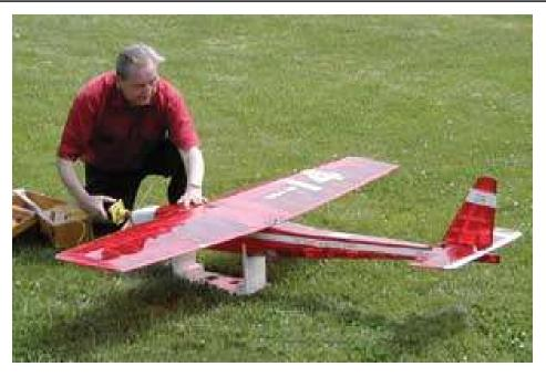
Legally blind model aircraft designer and experimenter Maynard Hill with model "Spirit of Butt's Farm" which crossed the Atlantic in August 2003, flying 1,920 nautical miles in 37 hours. It landed with 1.8 oz of fuel left in the tank.
