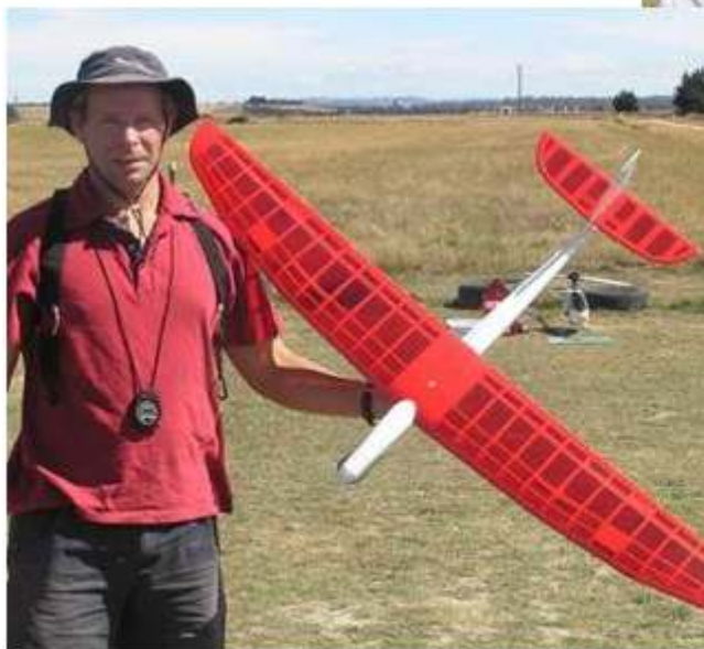
Mike Taylor with his own-design 400-powered glider. Has cobalt motor, ailerons and elevator.
